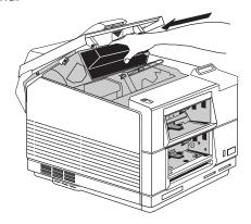
4 Grasp the tab protruding from the left side of the toner cartridge and flex it to break it loose.
